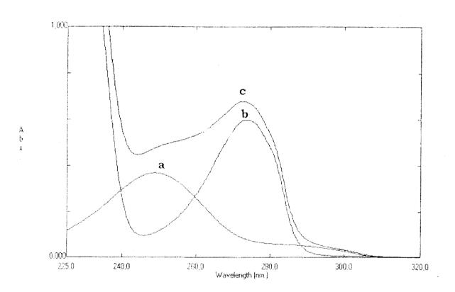
Figure 1. Zero-order absorption spectra of a) 3  $\mu$ g/mL solution of paracetamol, b) 20  $\mu$ g/mL solution of methocarbamol in methanol c) solution of 3  $\mu$ g/mL paracetamol + 20  $\mu$ g/mL methocarbamol mixture in methanol
